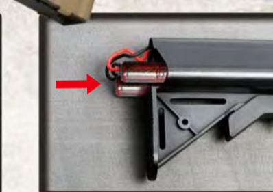
Insert the battery into stock.
