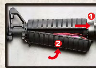
1. Pull the slip ring and hold. 2. Reinstall the lower handguard.
