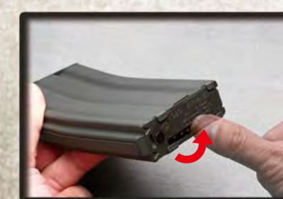
Close the cover plate then turn the gear until the sound changes.
